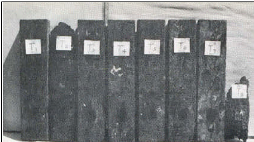
Fig. 2. Condition/appearance of medium density coconut wood panels After three years in sea water exposure. (L-R: T 1 , T 2 , T 3 , T 4 , T 5 , T 6 , T 7 and T 8 )
