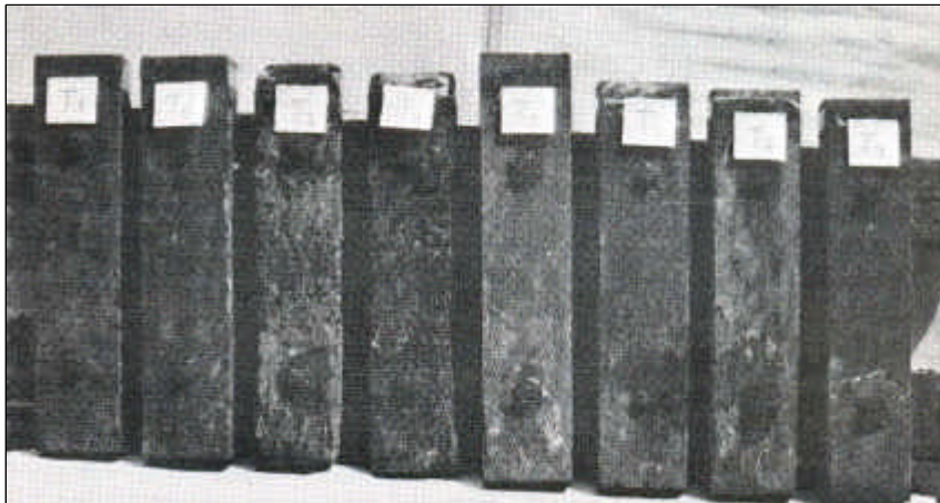
Fig. 1. Condition/appearance of high density coconut wood panels after Three years in sea water exposure. (L-R: T 5 , T 4 , T 2 , T 8 , T 3 , T 1 , T 6 and T 7 ).
