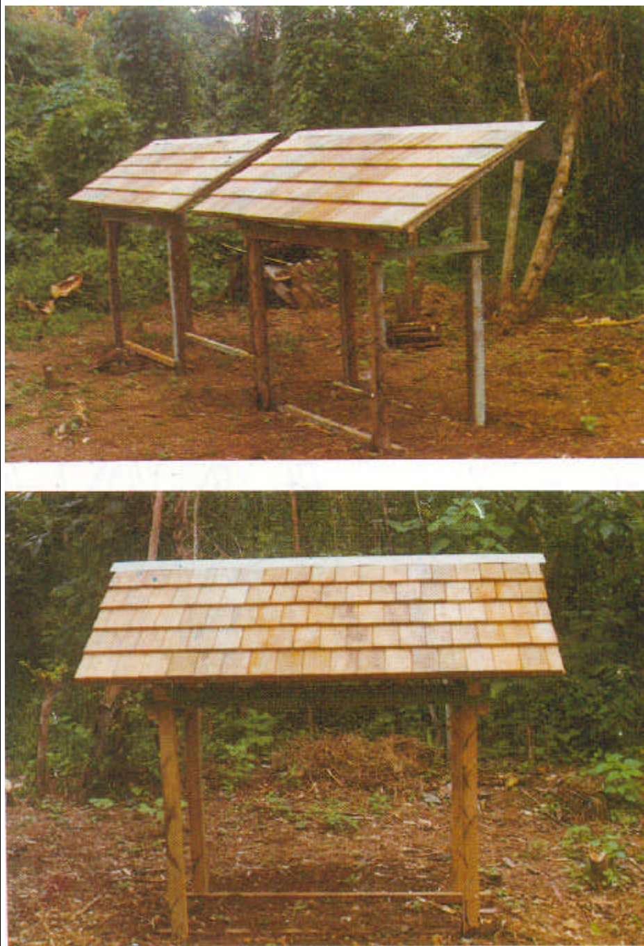
Figure 4. Coconut wood roof shingles exposed outdoors at the FPRDI “graveyard” area.
