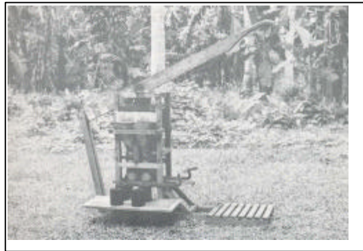
Figure 9. Densification molder for small coconut charcoal Briquettes production
