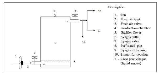
Figure 3. Coco peat gasification with updraft gasifier
