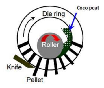
Figure 2. Mechanism of coco peat pelletizing
