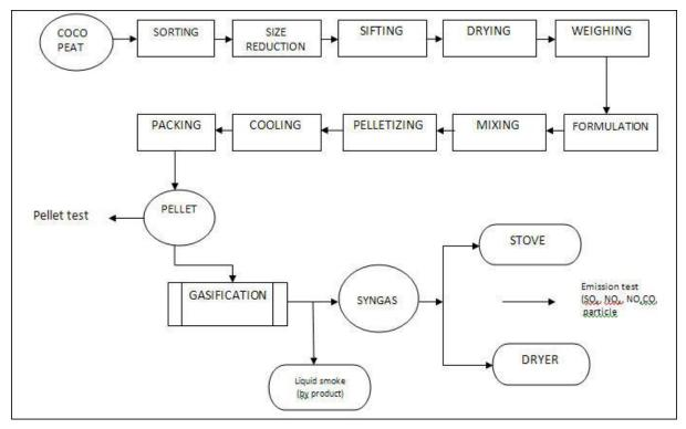
Figure 1. Flow process of coco peat production and test
