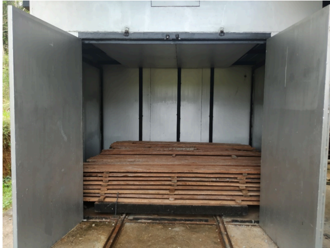
Plate 2. 25 mm thick coconut palm planks stacked in the convection Kiln
